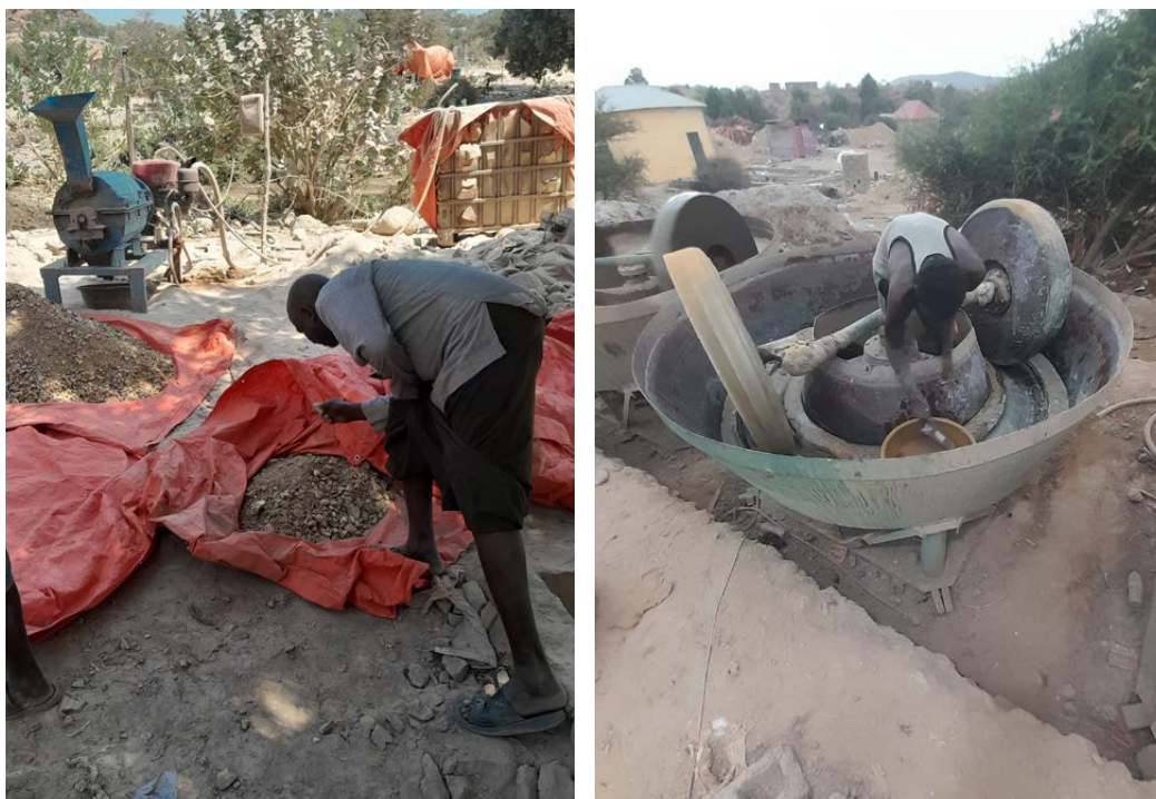
Left: A miner inspecting crushed quartz ore beside a small diesel-powered jaw, or hammer mill. Right: A labourer in Milxo who appears to be in the process of adding elemental mercury to a wet pan mill. (For further details on the processes used in Milxo, see Appendix 1.) Photos supplied
