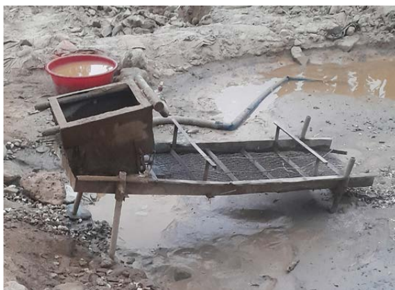
A rudimentary sluice box used to wash crushed ore or alluvial deposits manually. Photos supplied
