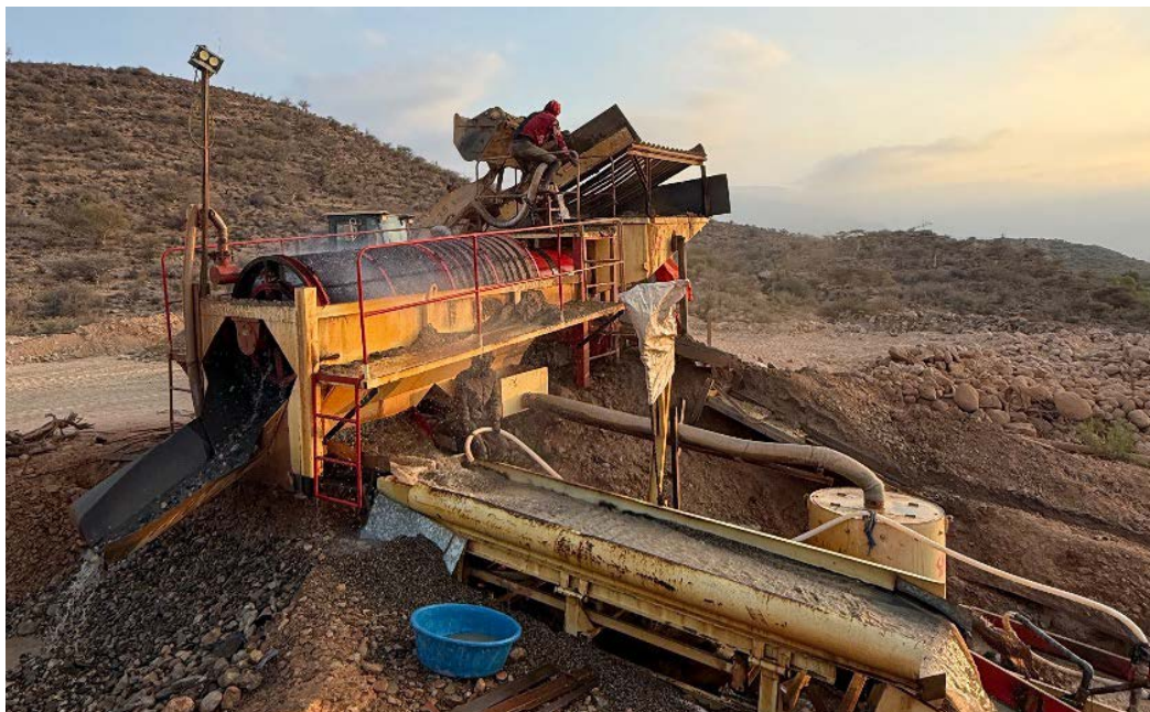
A trommel mill on the outskirts of Milxo, used to wash and separate gold-bearing ore. Photo supplied
