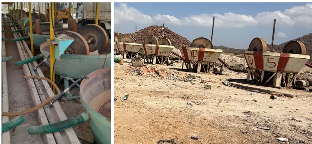
Wet pan ('Sudan') mills, used to grind crushed quartz into a slurry for mercury amalgamation.
