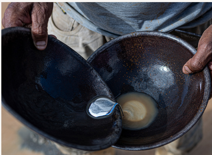
A miner amalgamates gold with mercury in Madre de Dios, Peru. This extraction method has contaminated rivers and caused severe health impacts in indigenous and riverine communities. © Ernesto Benavides/AFP via Getty Images
