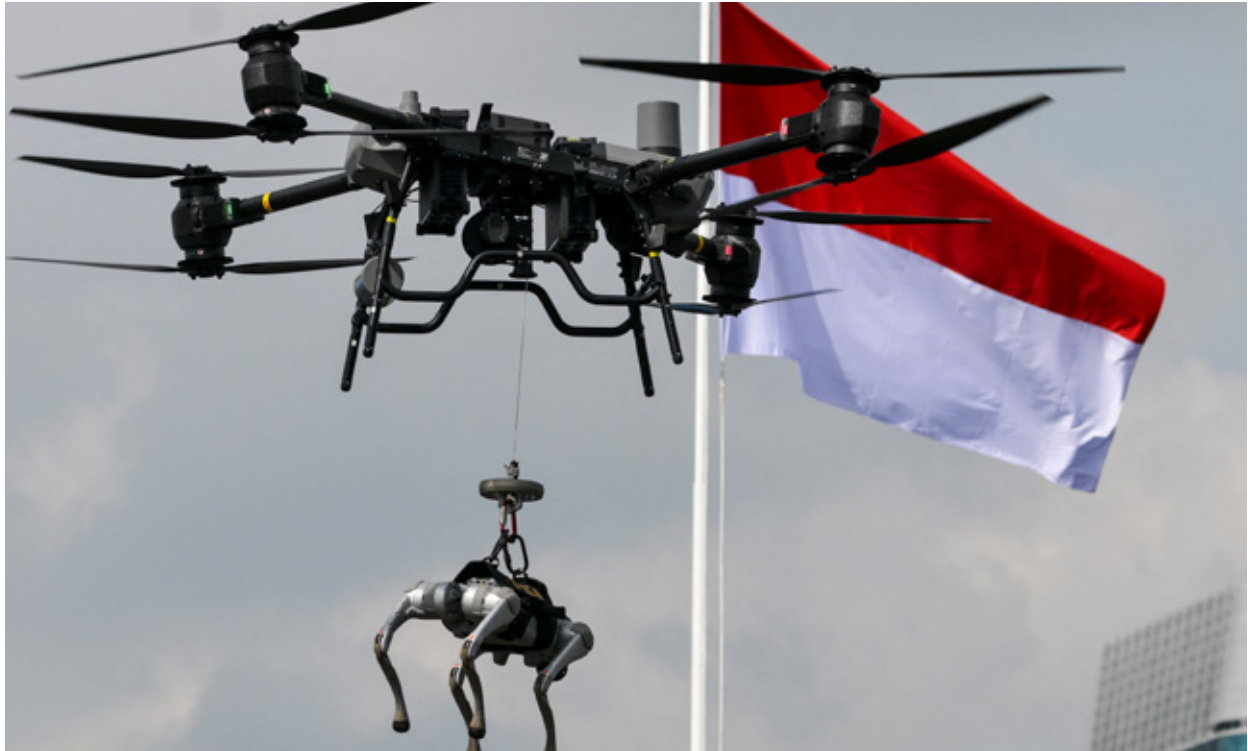
Land drones, like this dog reconnaissance drone, can be delivered by aerial platforms to desired locations. Conversely, land drones can also deliver aerial drones. © Bay Ismoyo/AFP via Getty Images
