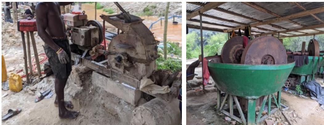
A diesel-powered rock crusher (left) and wet pan mill (right) of Chinese origin. Both machines are commonly used in the Western region. Photos: GI-TOC
