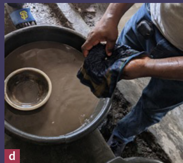
Concentrate and mercury are combined to form an amalgam ball, and processors use a cloth to remove excess water.
