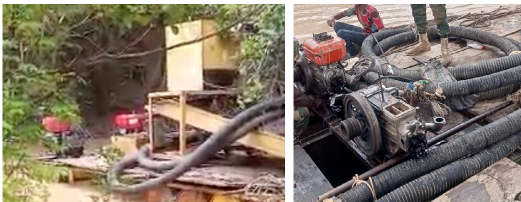
A floating platform equipped with changfa engines imported from China. These highly mechanized systems are exerting very damaging impacts on the environment. Photos: GI-TOC
