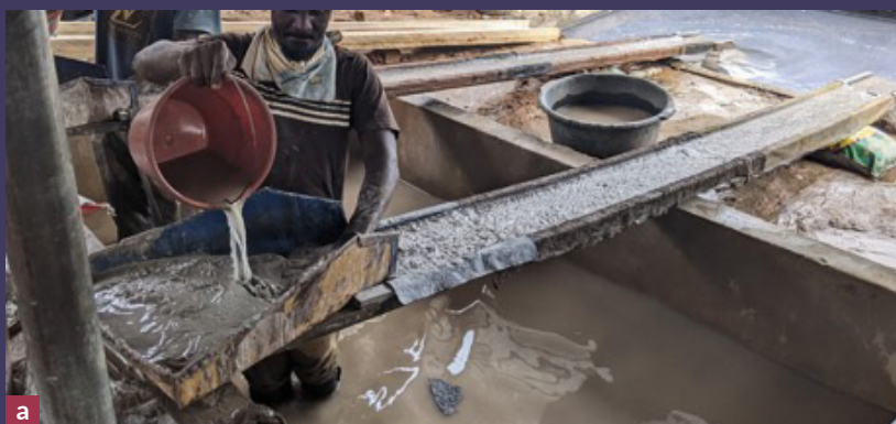
A sluice to capture concentrate, also known as 'mud'.
