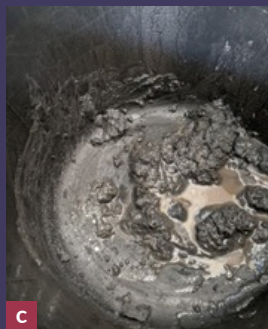
The mercury is mixed with ore concentrate.
