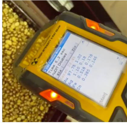
An X-ray fluorescence spectroscopy (XRF) scanner being used to test the purity of artisanally smelted gold bars (left) and nuggets (right). In this case, the gold nuggets were found to be just under 98 per cent pure. Photos: Stills from video supplied by source
