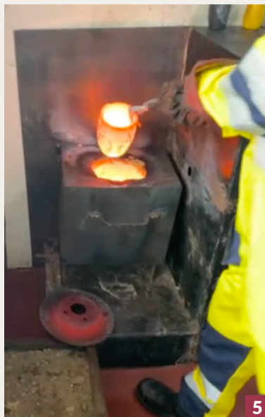
A fire assay of a doré bar carried out at the artisanal facility in Nairobi's Lavington neighbourhood. Flux – typically a combination of borax and sodium carbonate – was added to the molten gold during steps 3 and 4. Photos: Stills from video supplied by source
