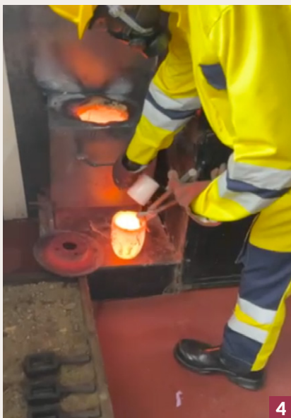
A fire assay of a doré bar carried out at the artisanal facility in Nairobi's Lavington neighbourhood. Flux – typically a combination of borax and sodium carbonate – was added to the molten gold during steps 3 and 4. Photos: Stills from video supplied by source
