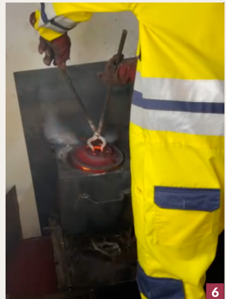
A fire assay of a doré bar carried out at the artisanal facility in Nairobi's Lavington neighbourhood. Flux – typically a combination of borax and sodium carbonate – was added to the molten gold during steps 3 and 4. Photos: Stills from video supplied by source
