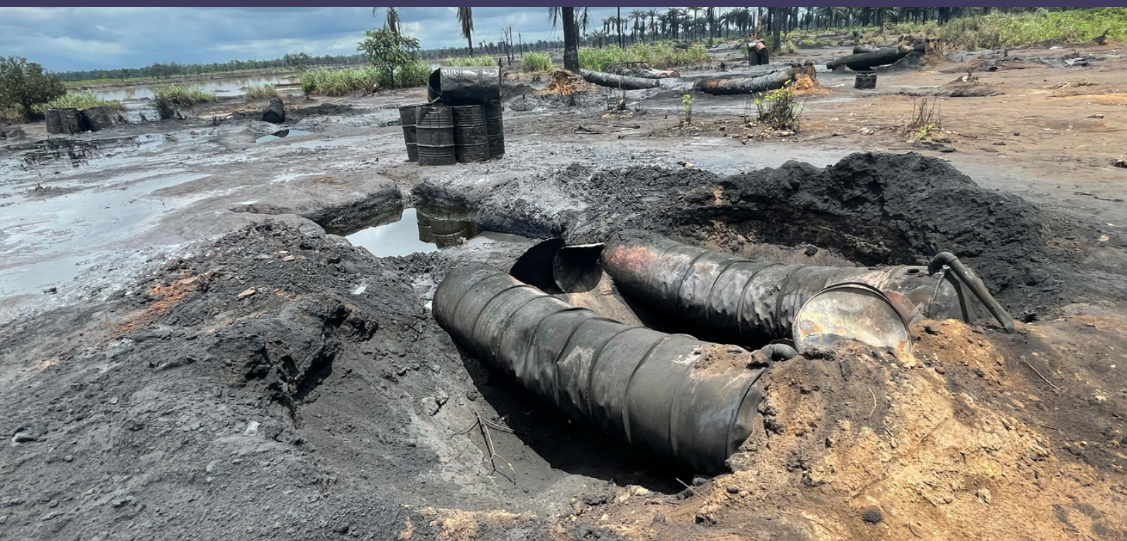
Boiling drums used to refine crude oil at an illegal oil refining site in Egbema, Rivers State, August 2021.
