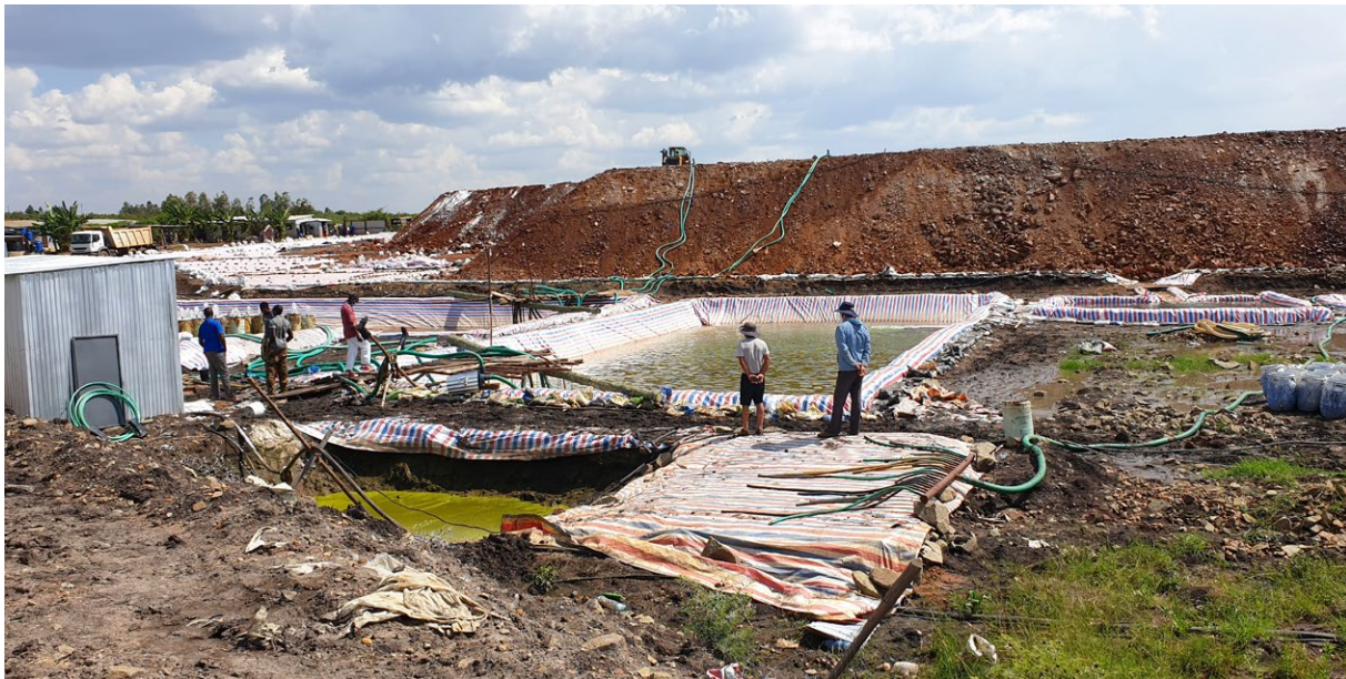
A gold leaching site in Migori county, Kenya, that uses sodium cyanide to extract gold from waste products of previous gold mining. Sodium cyanide can contaminate water sources if the proper precautions to secure leaching sites are not followed. Photo: Manuel Odeny
