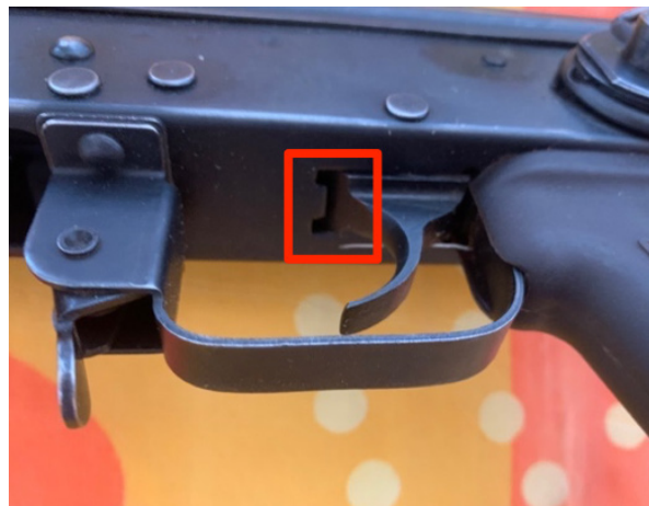
The 'double notch' at the base of the rifle's trigger is distinctive of Chinese manufacture.
