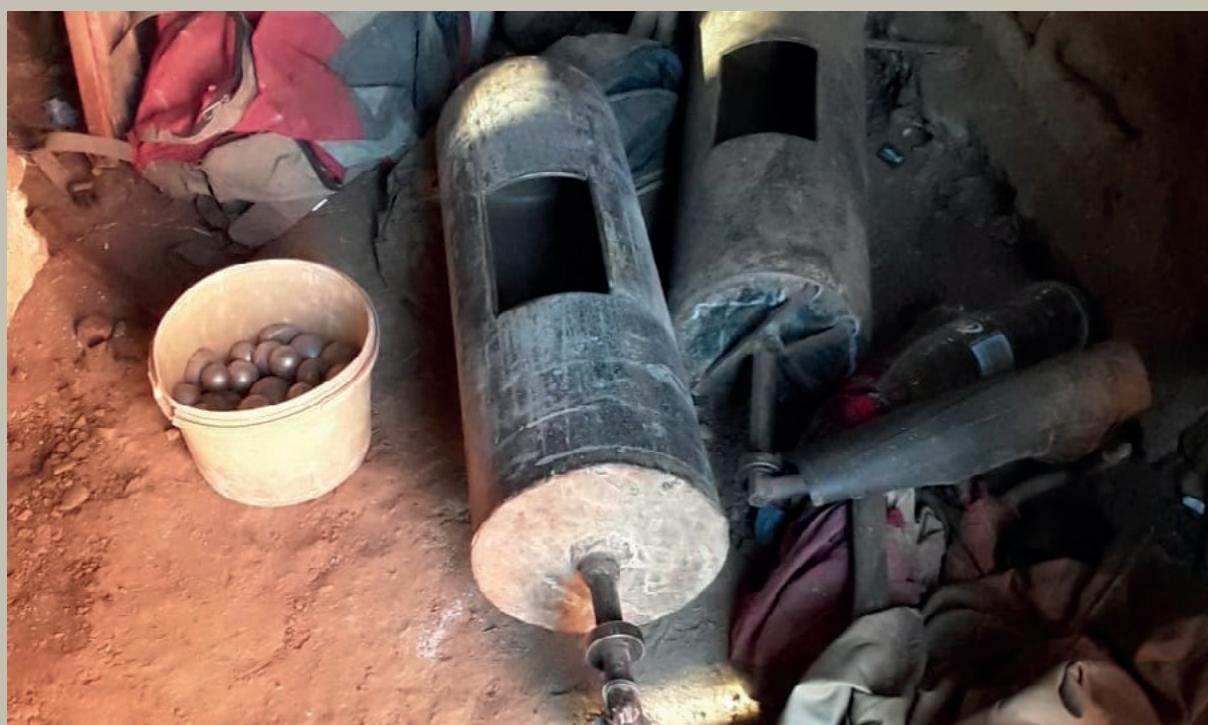
Simple equipment for processing gold ore. The cylindrical pieces of equipment are known as phendukas , which along with the ball bearings (pictured in the bucket), are used to break up the rock before processing and extracting the gold. PHOTOS: Supplied
