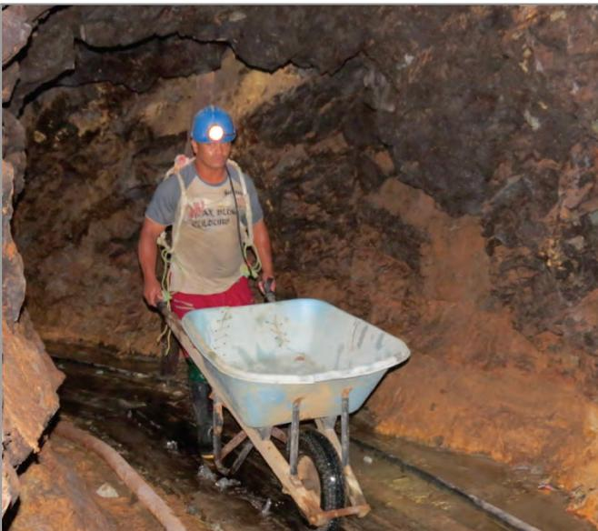
This is one of the most common techniques in the Chocó area. It is an excavated pit, with walls held by wooden poles. The depth of the holes depends on the distance of the place where the gold and the platinum are located, but can be up to 15 meters deep. Photograph by Oro Verde.
