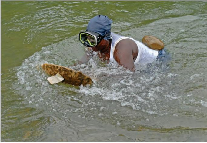
This artisanal method used in prolonged summer periods, when river levels drop. The gold is located at the bottom of the river and the miner makes successive dives to take out the gold and platinum containing material which is washed using a pan. Photograph by Kike Arnal.
